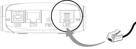
A top-down view of the SAGEM F@st modem. The ports are labeled USB, ETH, PWR, and LINE. A telephone line lead is being inserted into the LINE port, which is circled in red. An arrow points from the lead to the port. |
