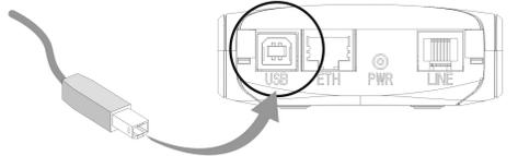
A top-down view of the SAGEM F@st modem. A USB cable is being inserted into the USB port, which is circled in red. An arrow points from the cable to the port.                                                          |
