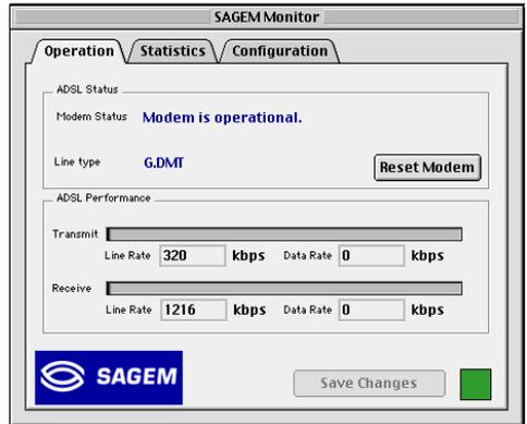
The content of the "Operation" tab in the diagnostics screen is explained below.
