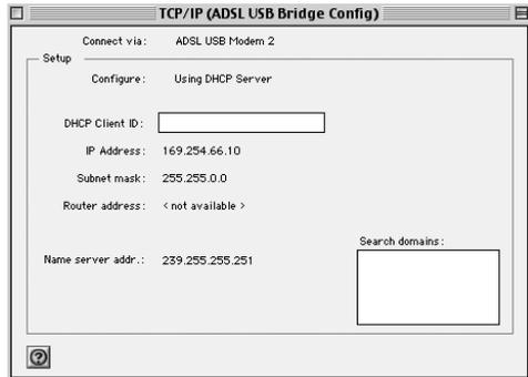
**Note:** The **Connect via:** and **Configure:** fields should respectively contain **ADSL USB Modem xxx** and **Using DHCP Server**.
