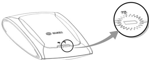
For this, use the power supply unit supplied with your modem<sup>1</sup>. When the modem is powered up, the PWR LED lights.
