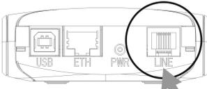
The line lead supplied in your pack should connect the modem to the connector provided on your splitter or to a telephone network adapter.
